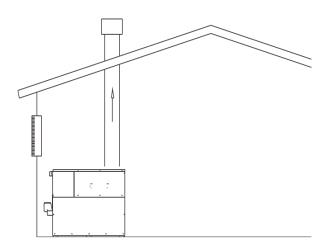
FIG. 6 Outside Combustion Air - Single Opening
